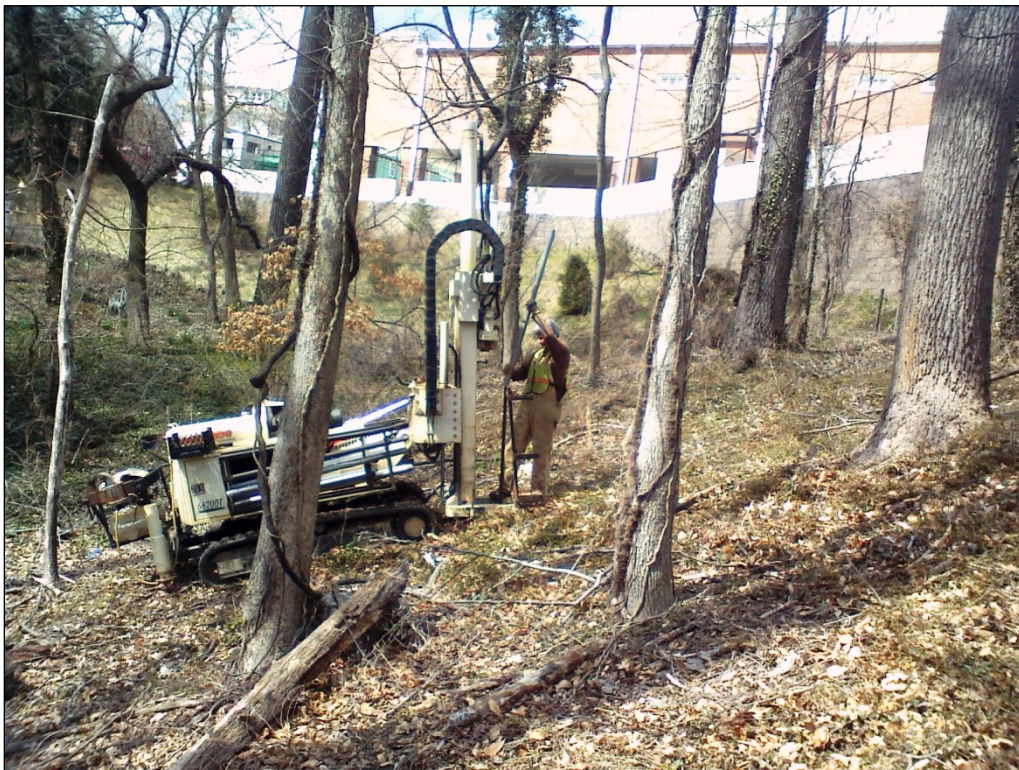
The Geoprobe track rig at sampling point TJ-GP-11, with the Takoma Park Volunteer Fire Department in the background.
