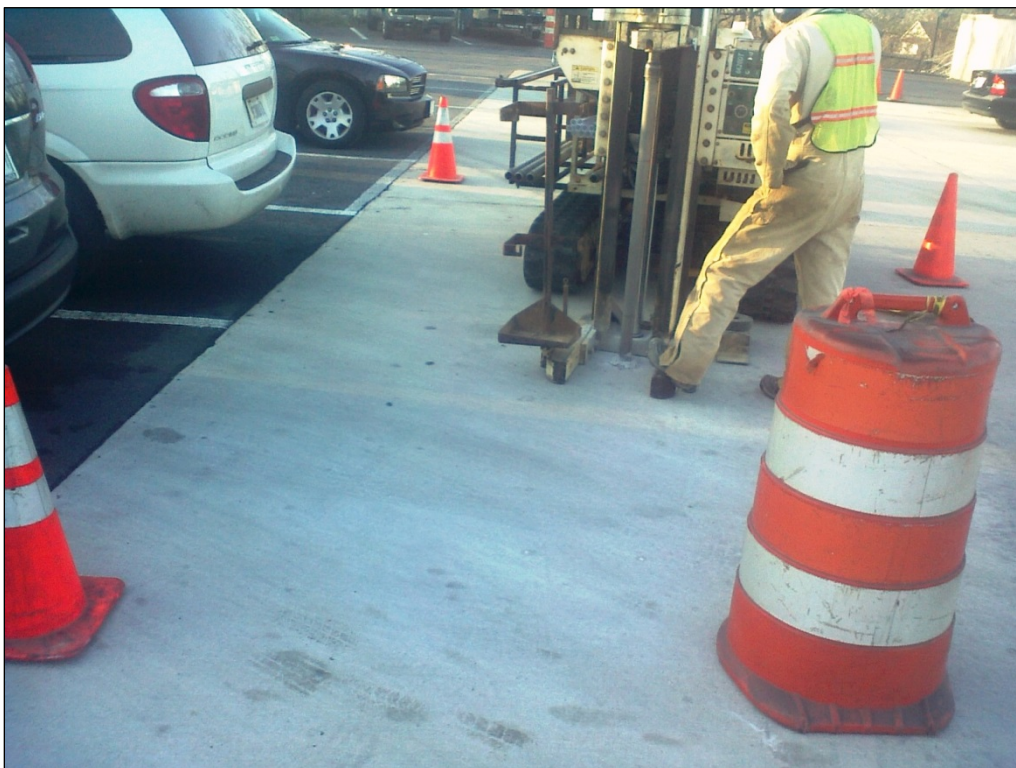
The Geoprobe track rig, with safety cones, at sampling point TJ-GP-01, cutting through the concrete pad.
