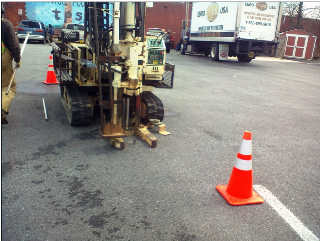
The Geoprobe track rig, with safety cones, at sampling point TJ-GP-05, with Takoma Park-Silver Spring Cooperative in the background.
