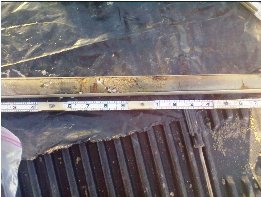
A representative view of a Geoprobe sample column in opened plastic tubing, from new sampling point TJ-GP-15.
