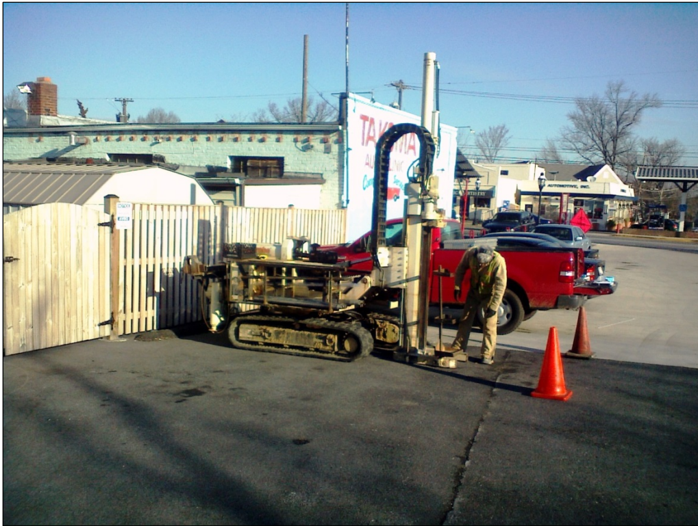
The Geoprobe track rig, with safety cones, at the new sampling point TJ-GP-15, with Takoma Auto Clinic in the background.
