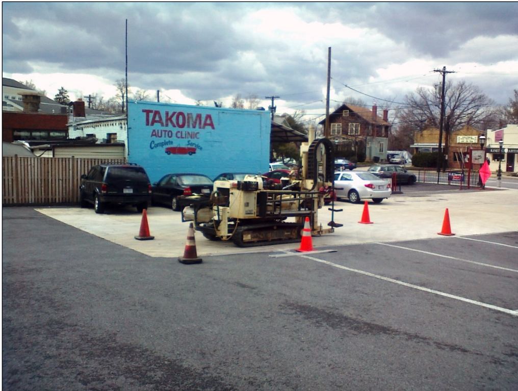
The Geoprobe track rig, with safety cones, at sampling point TJ-GP-04, with Takoma Auto Clinic in the background.
